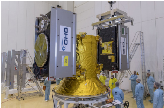
TWO OUT OF FOUR GALILEO satellites are attached to the dispenser pre-launch. (Photo: ESA)
