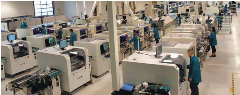
▲ FOUR SMT LINES continuously assemble, inspect, and test printed circuit boards.
