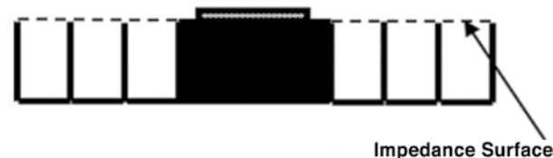
Fig.2 Cross-sectional view of the choke grooves structure
