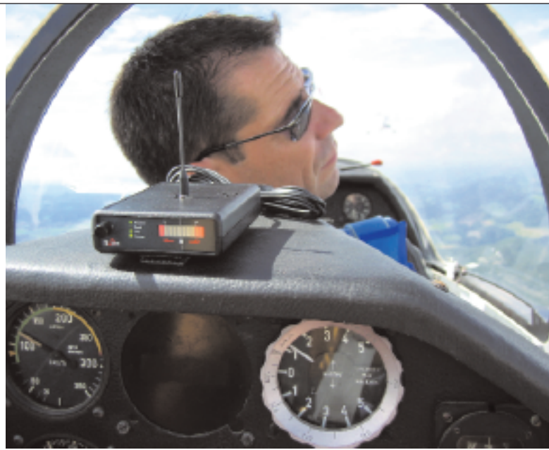
▲ THE FLARM SYSTEM mounted atop a glider pilot's instrument console, with the man serving as a second pilot or passenger
