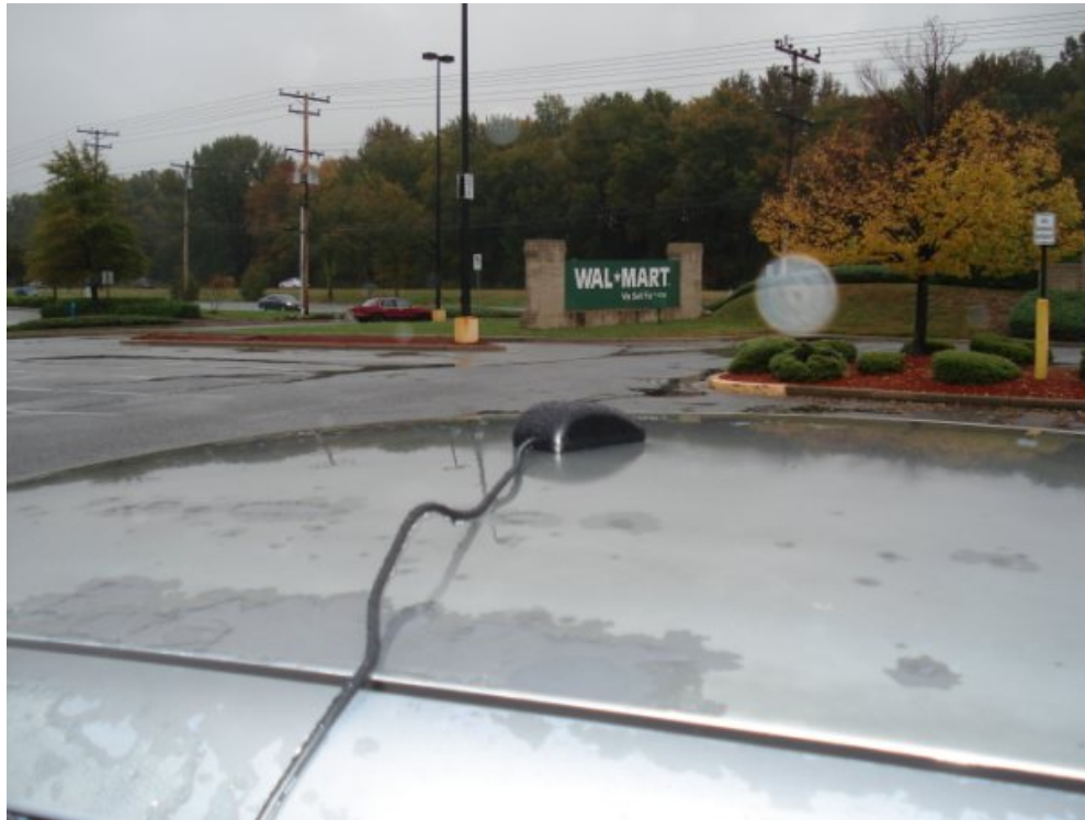
Figure 2: Antenna Mounting on Vehicle for GPS Received Power Measurement
